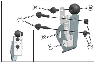
Install door lock ball (16) on the lever hole of the LH door lock (11) using M6x12 hex flange bolt (20), then install the LH door lock (11) on the LH door lock bracket (10) using two M6x25 hex flange bolts (22) and two M6 nuts (23).
