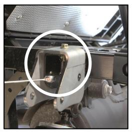
2. Install the bracket to the frame shock mount. Use (1x) M10x70mm bolt, (1x) 1-9/16" Lg. spacer and (1x) M10 lock nut.
