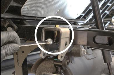
2. Install the bracket to the frame shock mount. Use (1x) M10x70mm bolt, (1x) 1-9/16" Lg. spacer and (1x) M10 lock nut.
