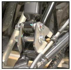
4. Tight all the hardware appropriately at this point. Use a 14mm and a 15mm wrench and socket.
