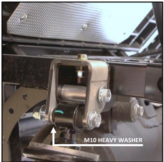
4. Tight all the hardware appropriately at this point. Start tightening with the M6 hardware.
