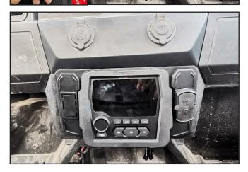
Position the radio (4) into the storage box, then install washers (13) and screws (11). Tighten the screws evenly, using caution not to over-tighten.
