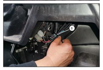
Connect the USB port (M) on the radio to the port (N) of the USB adapter cable (7).
