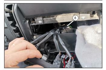
After radio debugging is completed, secure the radio cable and aerial (5) together with tie band (8).
