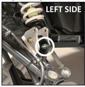
3. Connect the bottom of the shock to the new shock location on the brackets. Use (1x) M10-1.50 x 65mm bolt, (2x) M10 heavy washer and (1x) M10-1.50 lock nut. Put one washer on each side of the shock eyelet.
