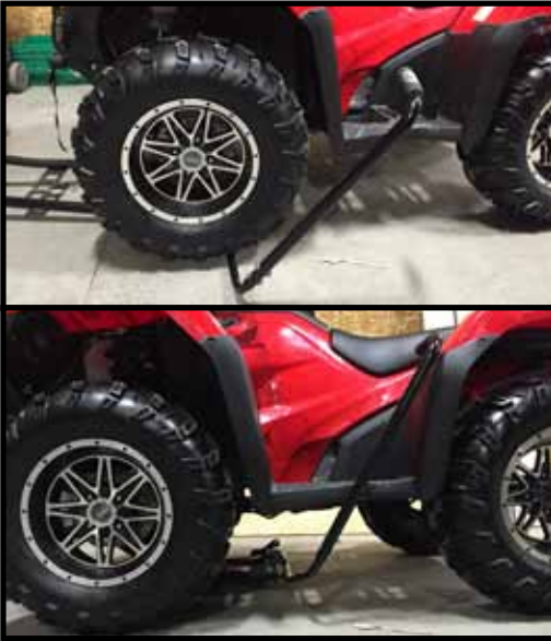
“Figure 12” Manual Lift Install
